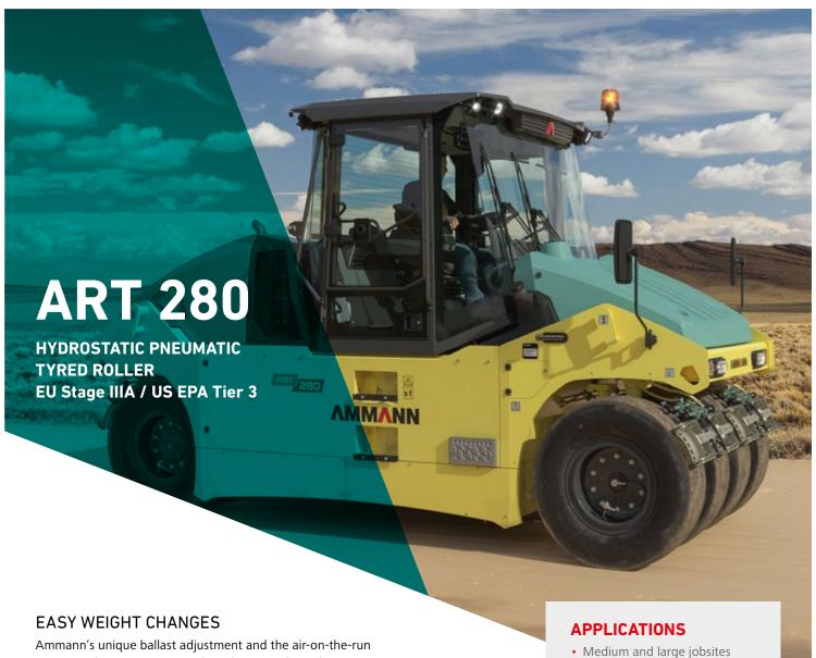
system make it easy to control machine weight and tyre pressure, the two main compaction factors. The modular, easy-load ballasting system enables weight to be adjusted from 9 tonnes to 28 tonnes in an hour – with the help of only a forklift. Brand new cab reduces sound and boosts operator comfort and safety. Improved serviceability keeps crews productive and maintenance costs to a minimum. The roller is powered by a EU Stage IIIA / US EPA Tier 3 Deutz engine with EGR and muffler.
