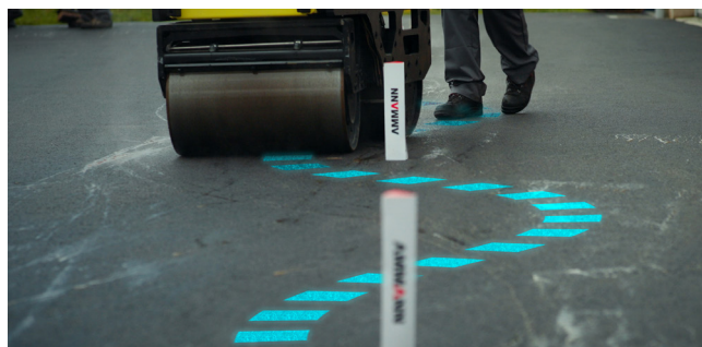
AWR 65-S Walk-Behind Roller with 15° steering angle
