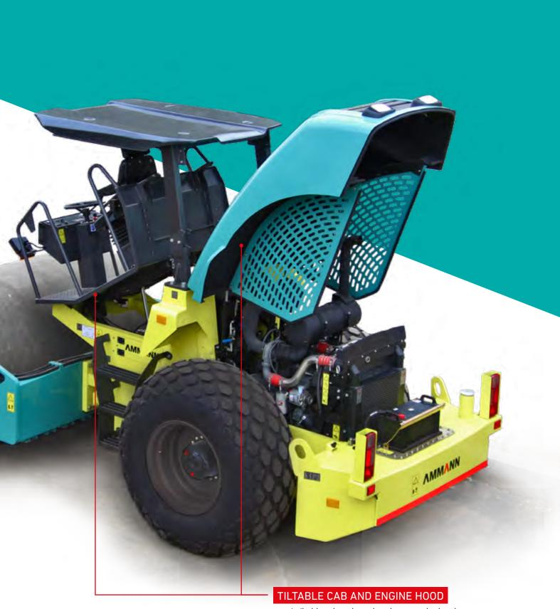
A tiltable cab and rear hood are standard and make hydraulic components easy to reach. The wide-opening hood provides outstanding access to the engine compartment, which can be reached from the ground.
