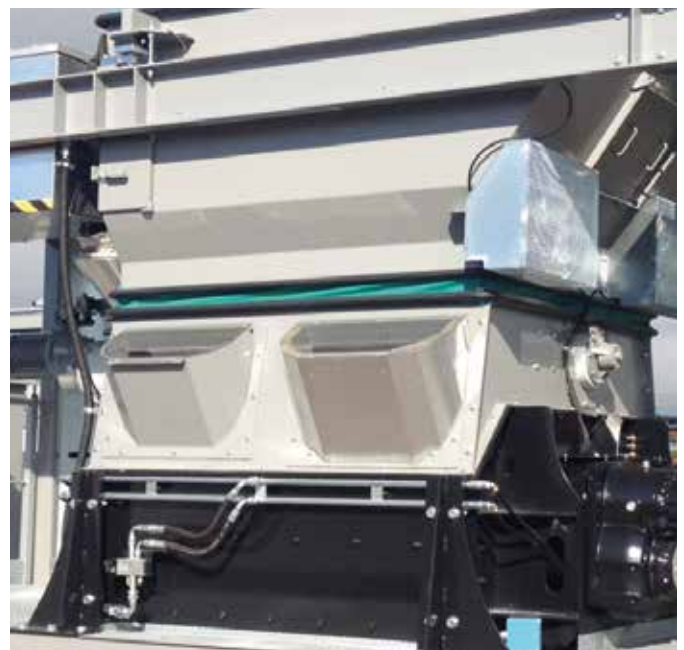
Mixer with integrated options for adding hot and cold recycling.
