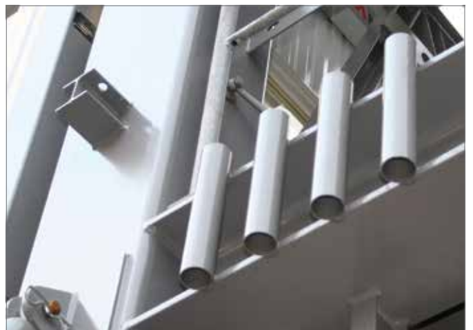
A place for everything: The majority of small components of the BlackMove II are securely stored for transportation. For example, the bolts for the telescopic mixing tower supports are located in special storage pockets.
