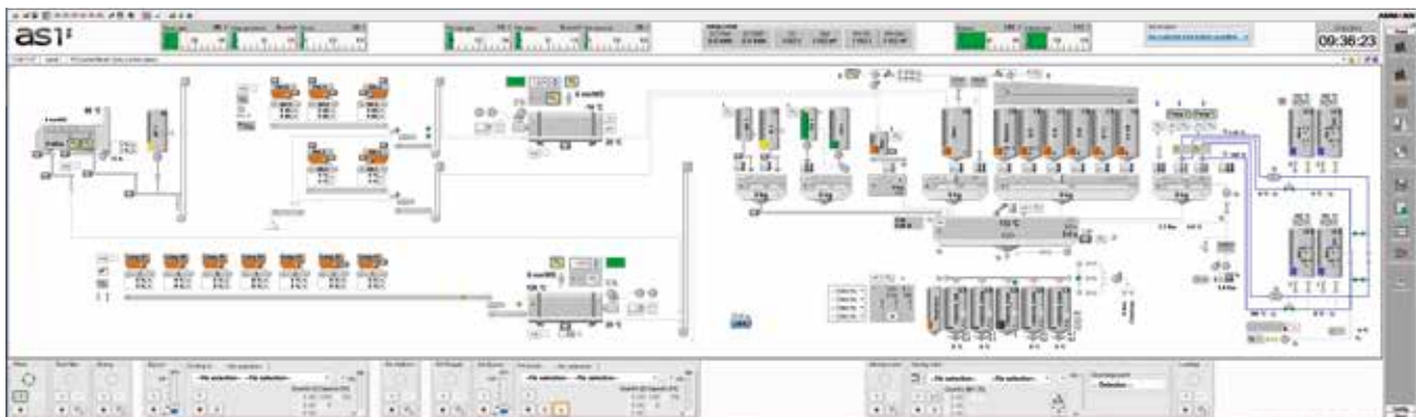
as1 control system for batch production.
