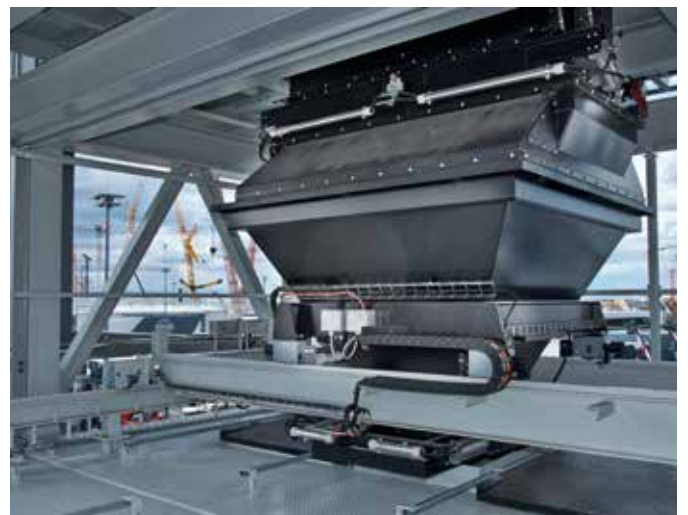
Encapsulated skip for reducing dust and smoke emissions.
