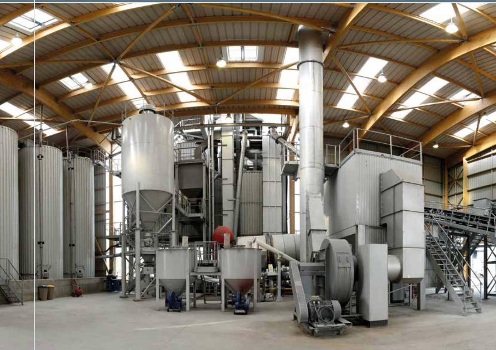
Photo above: Before cladding the mixing tower – the ContiMix is equipped with a recycling drum RAH100. Photo under: ContiMix fully clad (internal view).
