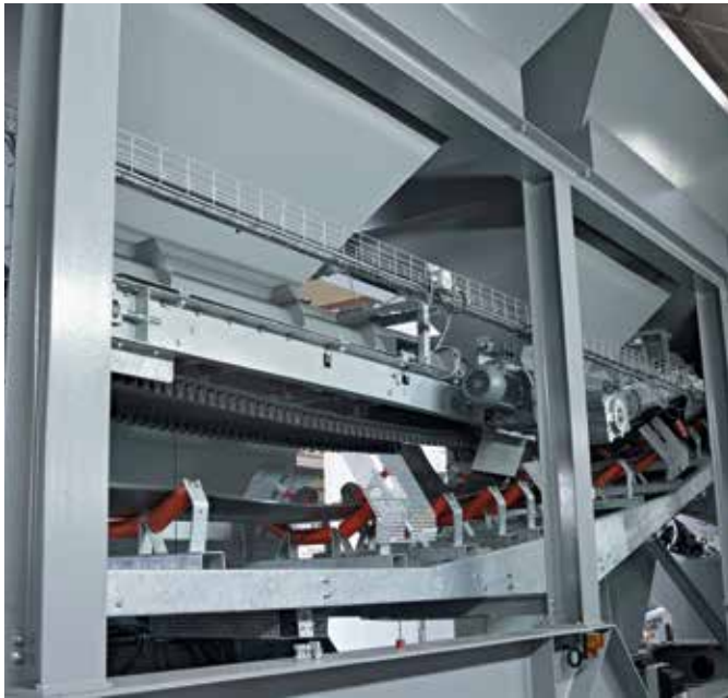
Cold feeders with gravimetric device.
