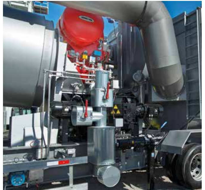
Drying drum with optimised efficiency high performance burner and the Amix twin-shaft compulsory mixer with adjustable mixing duration.
