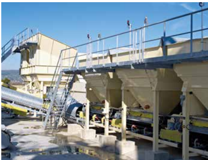
Cold feeders with indicator light and laser level control.
