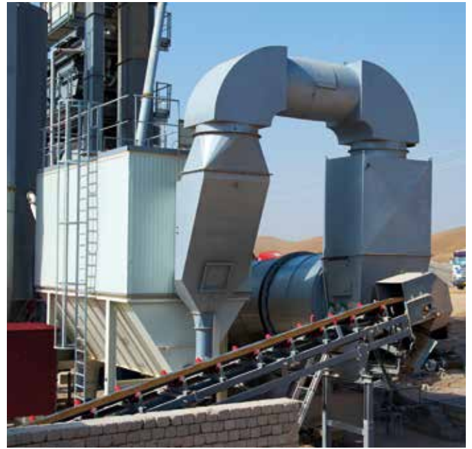
The highly accurate pre-separator reduces the load on the filter and increases the quality of the operator's own filler.
