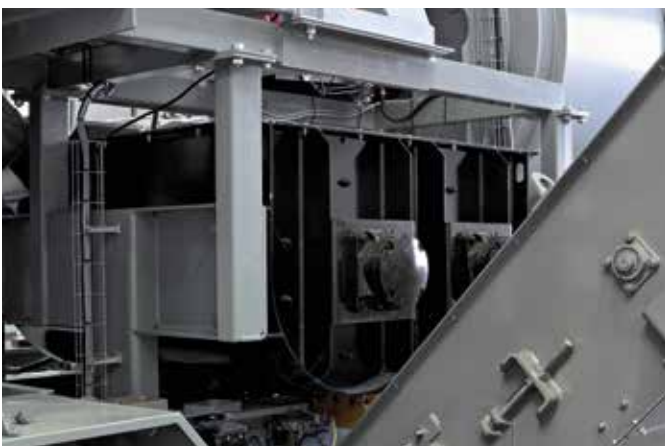
Amix twin-shaft compulsory mixer with adjustable mixing duration and a wivel-mounted drag slat conveyor with batcher. For high recycling addition to 40%, the extra long mixer is recommended.
