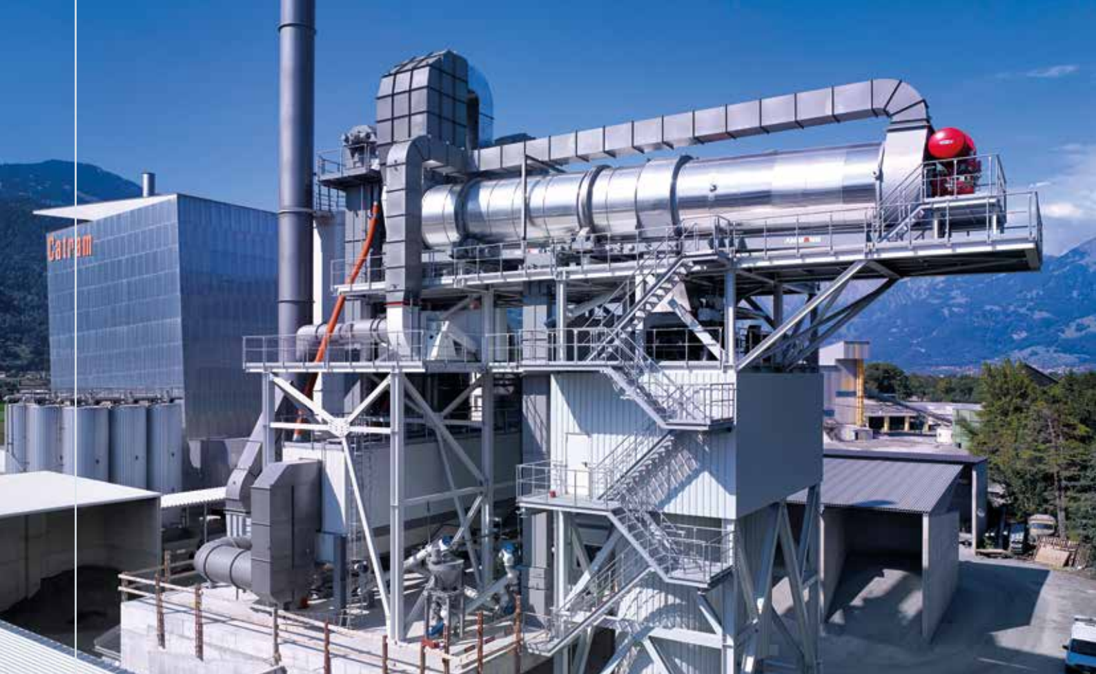
Photo above: Before cladding the mixing tower – the ContiMix is equipped with a recycling drum RAH100. Photo under: ContiMix fully clad (internal view).
