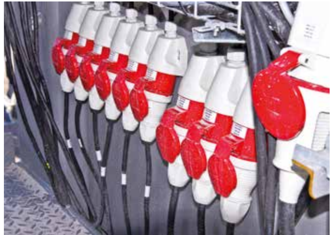
BlackMoveII: Electrical Connections: Rapid "plug and socket" connection, even to the main cable, mean that an electrician is not longer needed to erect the plant.
