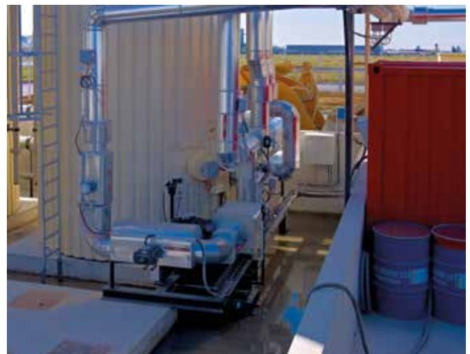
Precise dosing of the bitumen with the aid of the coriolis meter.
