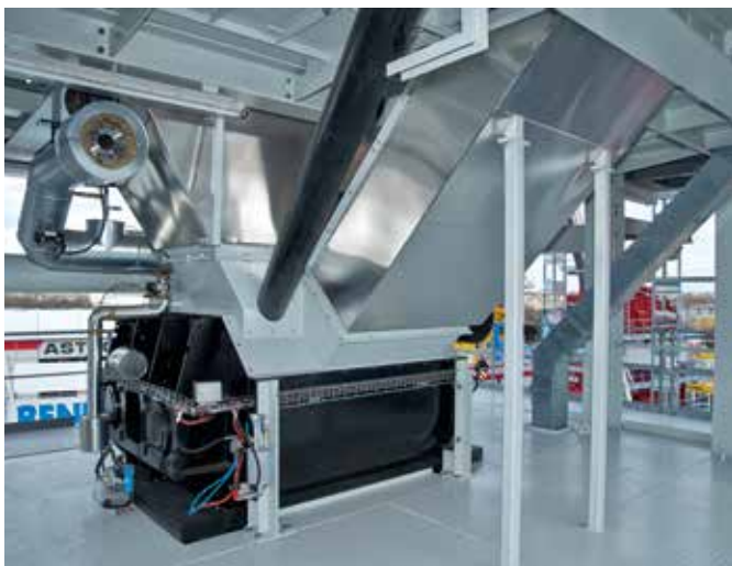
Amix mixer with aggregate chute.
