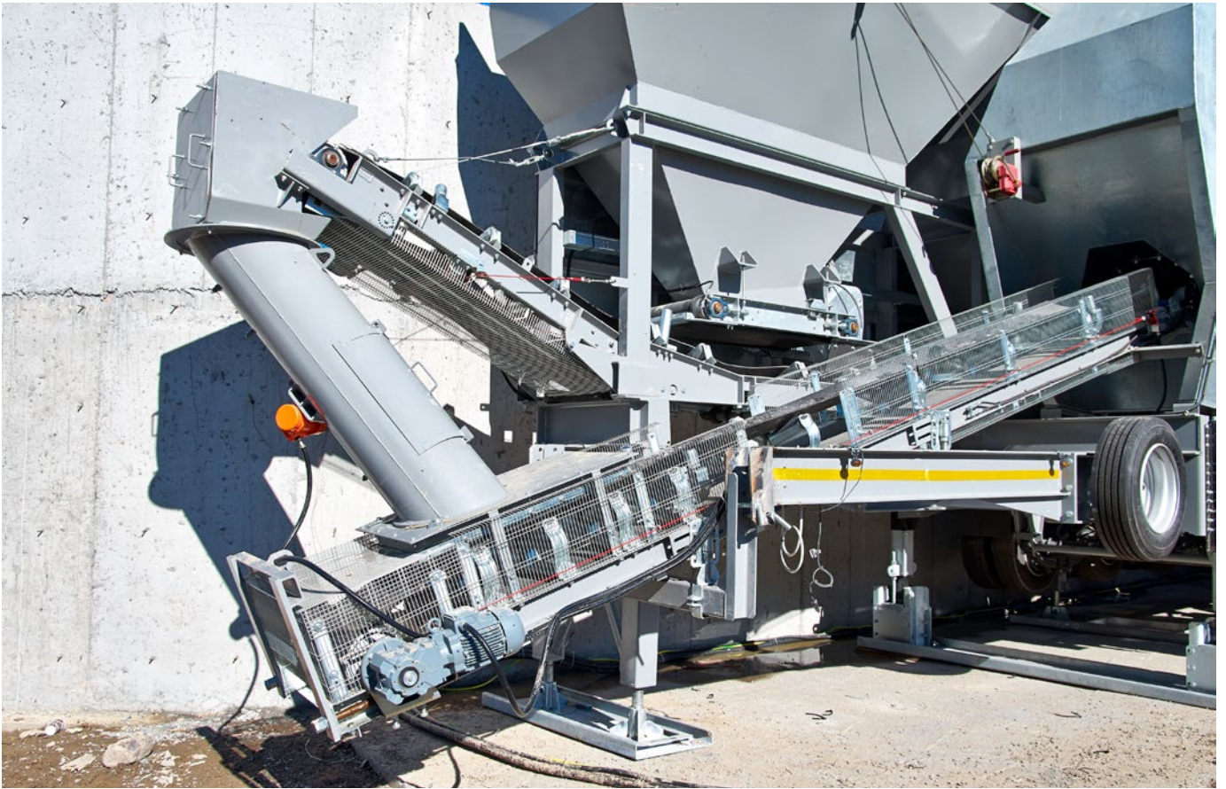
Compact and efficient: the transport of the different minerals from the cold feeder to the drying drum.
