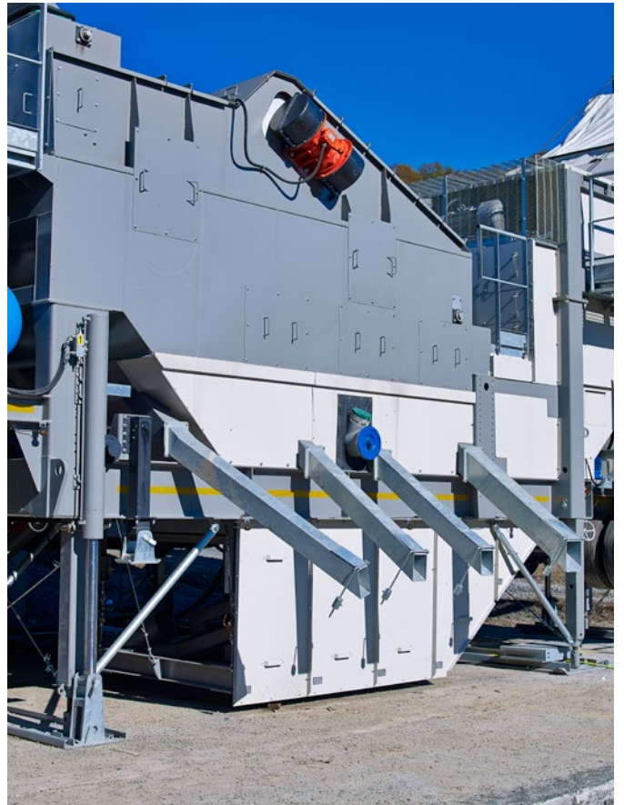
Trailer with a screen, hot aggregate silo and overflow channels as well as the bucket elevator to the mixer with integrated mineral scale.
