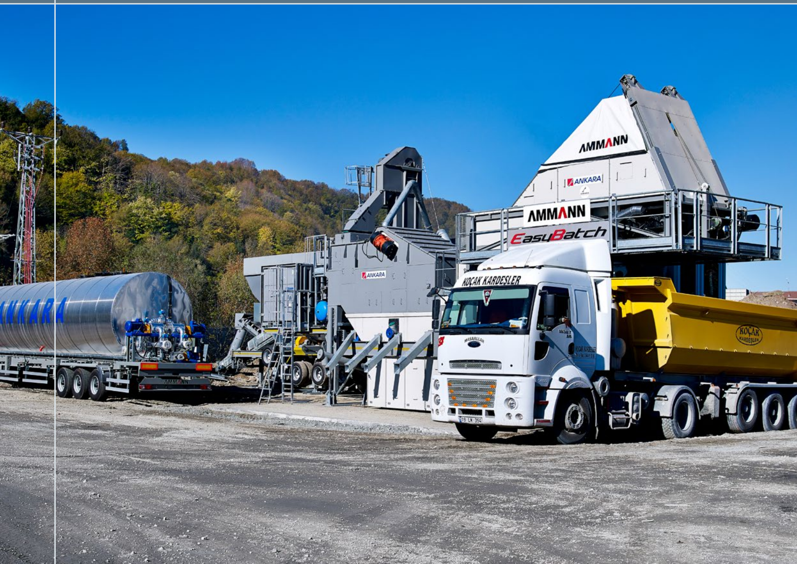
Photo under: The EasyBatch 140 can be equipped with a variety of features. In example with a mobile bitumen tank.
