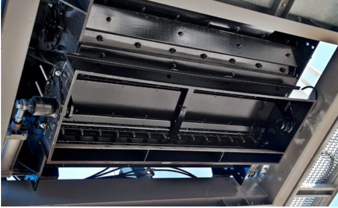
Direct loading: the mixer has generous outlet gates.
