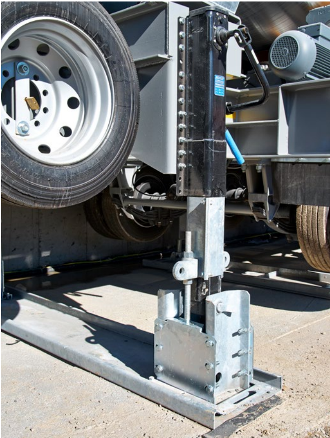
No special foundations are required for the erection. The erection site needs only be levelled and firm.
